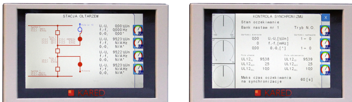
Fig. 7.1. Examples of screens of TS-20 synoptic plate
